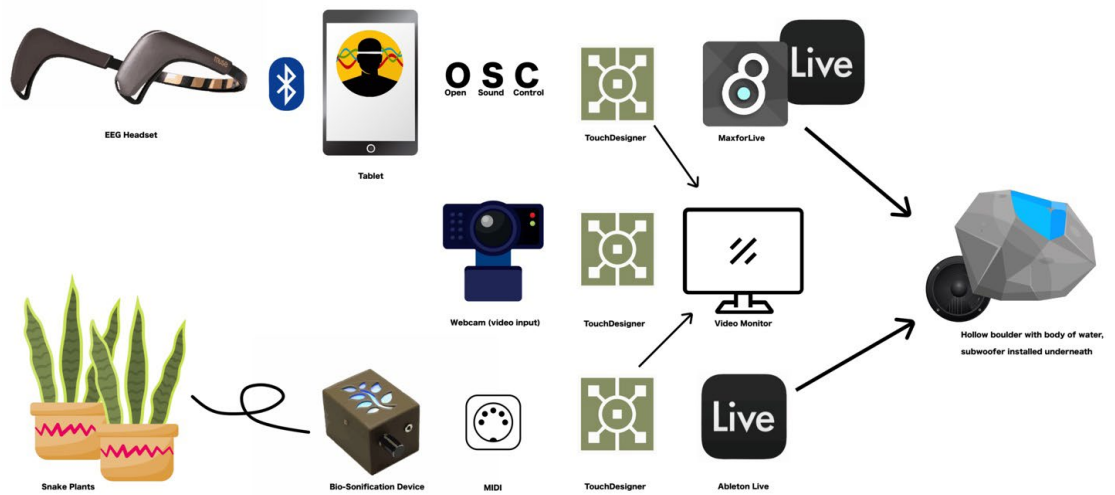
Fig. 3. Signal flow, stemming from three sources. Signal moves from left to right, generally.
