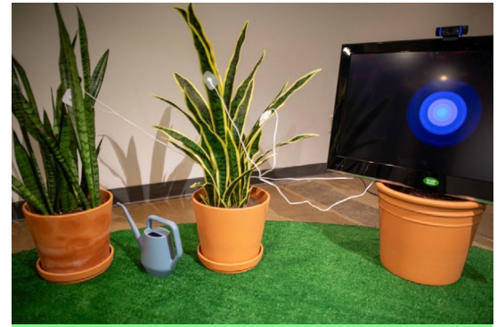
Fig. 2. Electrical conductivity sensors attached to plants. The monitor and webcam.
